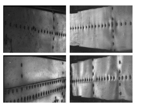
Aircrafts – a specific dataset containing 13075 grayscale images of the fuselage of aircraft structures, taken from 37 machines. The data has a resolution of 240x320 and is divided into two classes with corroded and non-corroded surfaces.
